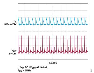
Figure 42. Switching Waveforms, Full Frequency Discontinuous Operation
