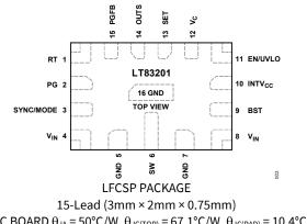
JEDEC BOARD  $\theta_{JA} = 50^{\circ}$ C/W,  $\theta_{JC(TOP)} = 67.1^{\circ}$ C/W,  $\theta_{JC(PAD)} = 10.4^{\circ}$ C/W DEMO BOARD  $\theta_{JA} = 33^{\circ}$ C/W,  $\Psi_{JT} = 1.7^{\circ}$ C/W EXPOSED PAD IS GND AND SHOULD BE SOLDERED TO PCB
