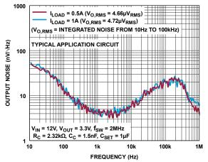
Figure 4. Noise Spectral Density vs. Load
