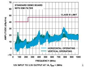
Figure 47. LT83201 Radiated EMI Performance (CISPR32 Radiated Emission Test with Class B Limits)
