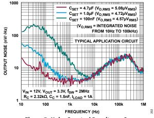
Figure 5. Noise Spectral Density vs. CSET
