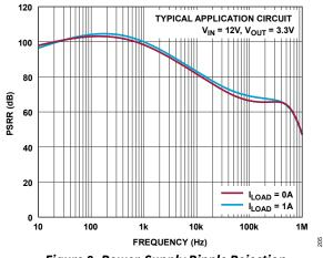
Figure 8. Power-Supply Ripple Rejection
