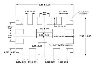
Figure 68. Tiny 15-Lead 3mm × 2mm LFCSP
