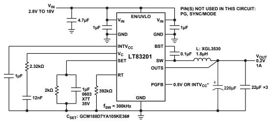
\*NOTE THAT APPLICATIONS WITH V<sub>OUT</sub> BELOW 0.5V WILL NOT BE ABLE TO USE THE POWER GOOD AND FAST START-UP FUNCTIONALITIES AND MUST TIE PGFB TO 0.5V or INTV<sub>CC</sub> TO DISABLE THESE FUNCTIONS CORRECTLY.
