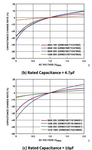
Figure 58. AC Voltage Characteristics for Different Capacitor Case Sizes
