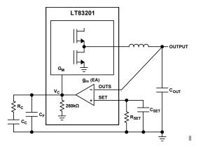
Figure 56. Model for Loop Response
