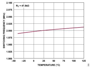
Figure 30. Switching Frequency vs. Temperature
