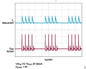
Figure 43. Switching Waveforms, Pulse-Skipping Discontinuous Operation
