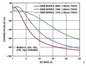
Figure 57. Capacitor Voltage Coefficient for Different Case Sizes
