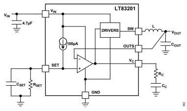
Figure 54. Adjustable Reference for Error Amplifier
