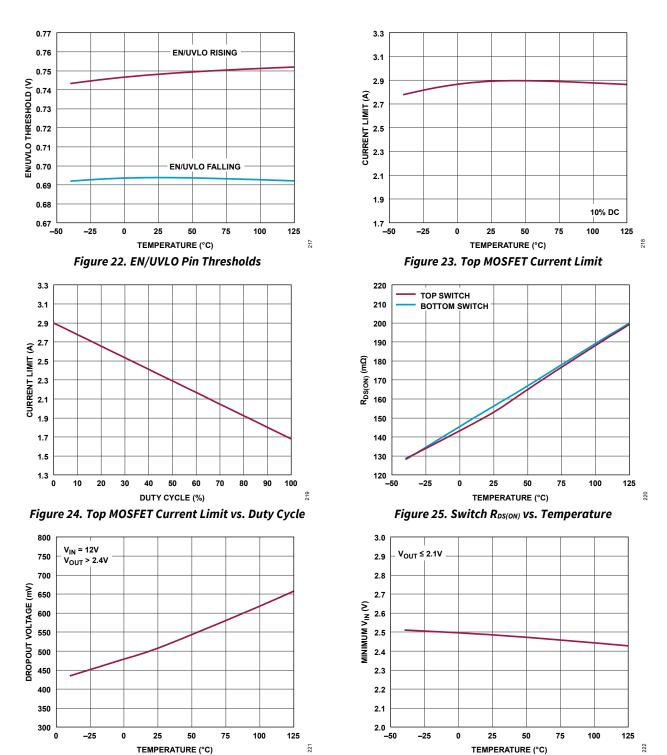
Figure 26. Dropout Voltage vs. Temperature
