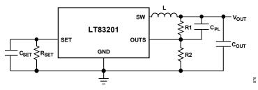
Figure 55. Configuring the LT83201 for Output Voltages above 13V
