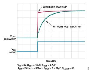
Figure 35. Start-Up Time with and without Fast Start-Up Circuitry for Large CSET
