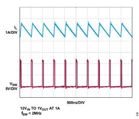
Figure 41. Switching Waveforms, Full Frequency Continuous Operation
