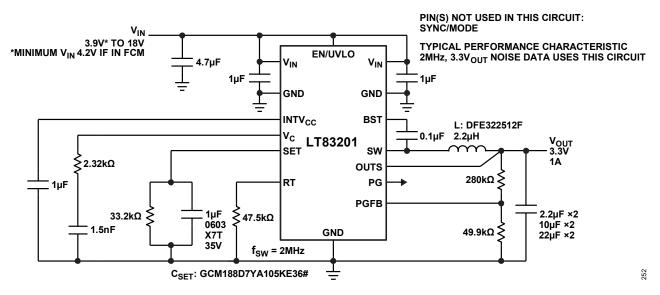
Figure 62. 3.3V 1A 2MHz Step-Down Converter with High Bandwidth, Soft-Start, Fast Start-Up and Power Good
