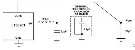
Figure 49. Additional Output Ripple Filtering Using Feedthrough Capacitors
