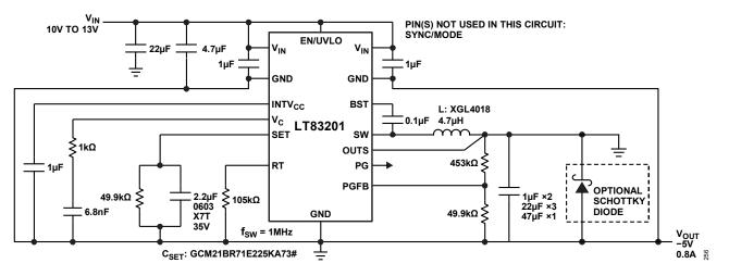
Figure 66. Negative 5V 0.8A 1MHz Step-Down Converter with Soft-Start, Fast Start-Up and Power Good
