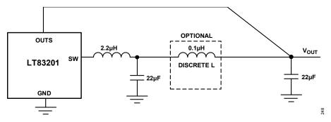
Figure 50. Additional Output Ripple Filtering Using a Second LC Filter
