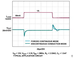
Figure 52. Load Step Transient Response with and without FCM
