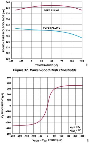
Figure 39. Error Amp Output Current
