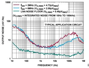
Figure 6. Noise Spectral Density vs. Switching Frequency
