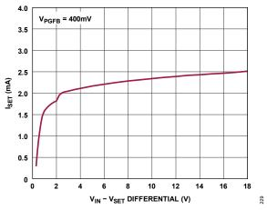
Figure 34. ISET During Start-Up with Fast Start-Up Enabled (vs. VIN - VSET Differential)
