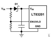
Figure 59. Reverse V<sub>IN</sub> Protection
