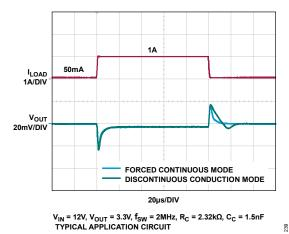
Figure 45. Transient Response: Load Current Stepped from 50mA to 1A
