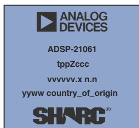
Figure 8. Typical Package Marking (Actual Marking Format May Vary)
