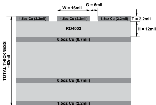
Figure 37. Evaluation Board Stackup
