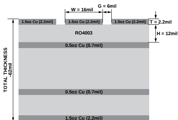
Figure 40. Probe Matrix Board Stackup, Cross Sectional View
