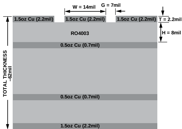
Figure 23. Evaluation Board Cross Sectional View
