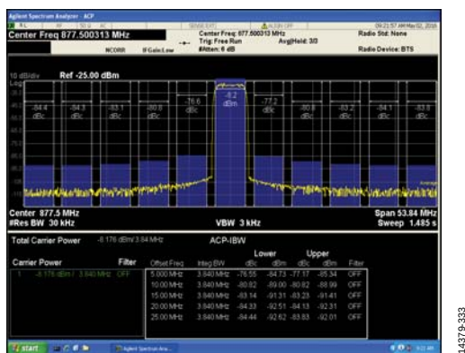
Figure 25. Single-Carrier W-CDMA at 877.5 MHz
