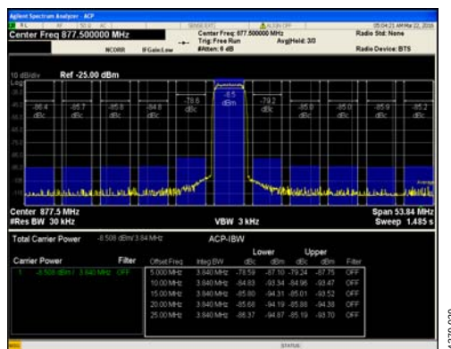
Figure 84. Single-Carrier W-CDMA at 877.5 MHz
