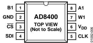
Figure 6. AD8400 Pin Configuration
