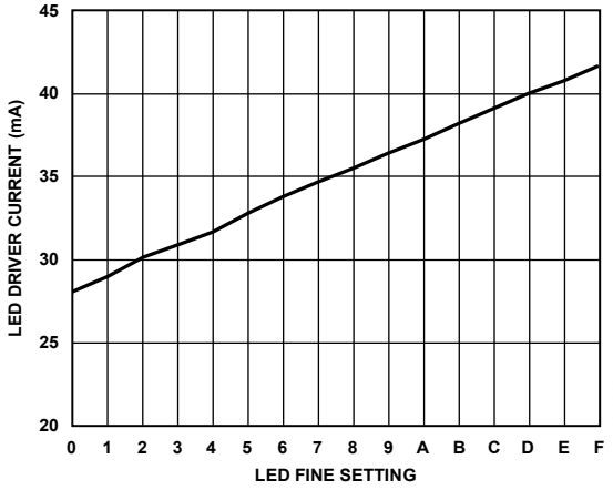
Figure 14. LED Driver Current vs. LED Fine Setting (Coarse Setting = 0x0)
